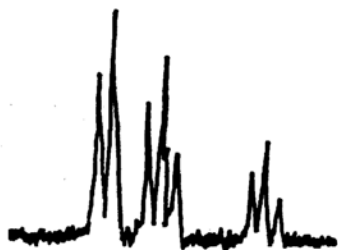
Fig. 1. The spectrum in the region of aromatic protons of the carbanion produced from 1,1-diphenylethylene in contact with excess potassium sodium alloy in THF. Applied magnetic field increases from left to right, at 60 Mcps.
